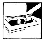
Run the washer through a complete cycle with one cup of detergent to clean out the antifreeze.
